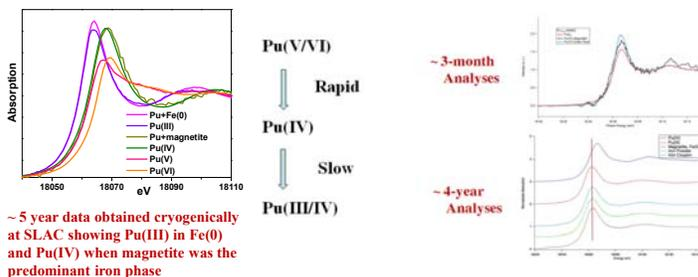
~5 year data obtained cryogenically at SLAC showing Pu(III) in Fe(0) and Pu(IV) when magnetite was the predominant iron phase
