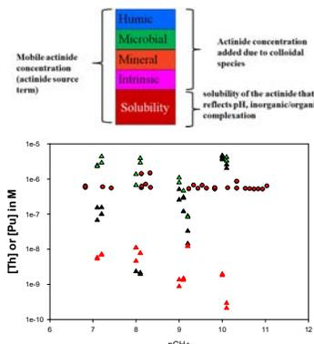
Comparison of Th (red circles) and Pu (triangles - green unfiltered, black 0.2 micron filtered, and red 30K-filtered) Solubility Data
